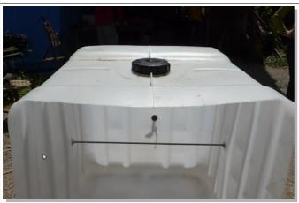
To stabilize the floating drum add a stainless steel threaded bar with two nuts, waver and rubber ring on each side. Make the bar a bit shorter, that the tank is pulled together (2").
