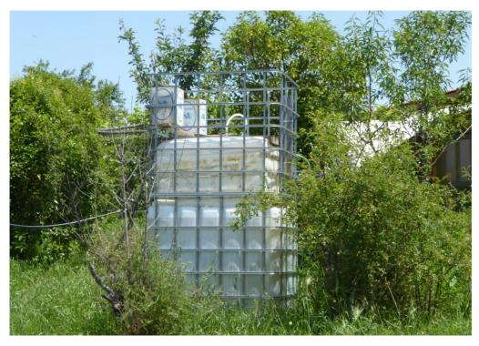
ARTIBC is a an ARTI Style system using two IBCs (International Bulk Container). It was developed by Solar CITIES Martin Funk, TH Culhane and Nick Chase in 2015 in Tamera. It's main purpose is gas storage.
