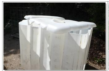
Lower IBC: In order to have a bucket within a bucket, cut the top of one IBC right below the curve.
