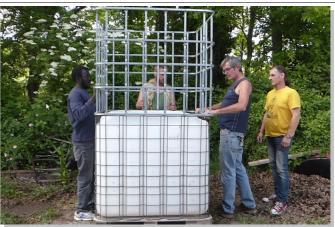
Then put the second cage on the top of the lower and fix it with cable stripper or pipe clamps.
