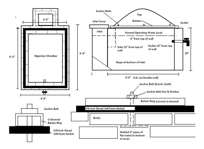
2 cu.m. Inflatable top plug-flow biogas digester
